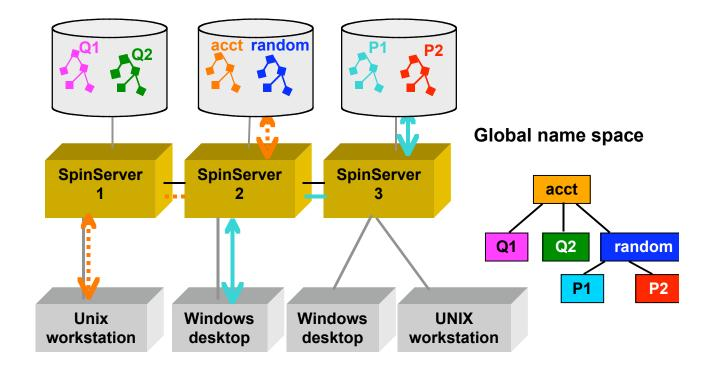
This architecture allows the constructing of a scalable cluster, but it requires the standardization of various intra-cluster protocols to allow the construction of heterogeneous clusters, with components provided by different vendors. Note that we expect that support for protocols other than NFS arriving at the user side of the SpinSever cluster will be required, since most NFS servers sold today also include support for protocols such as CIFS at a minimum.
