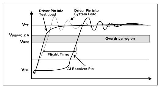
Figure 12-5. Measuring Nominal Flight Time
