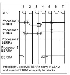
Figure 8-1. BERR# Protocol Mechanism
