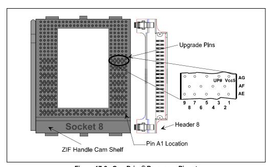
Figure 17-2. OverDrive® Processor Pinout
