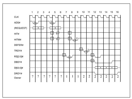
Figure 5-2. Response Responsibility Pickup Effect on an Outstanding Invalidation
