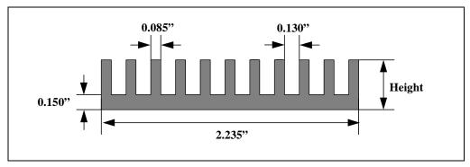
Figure 14-4. Analysis Heat Sink Dimensions
