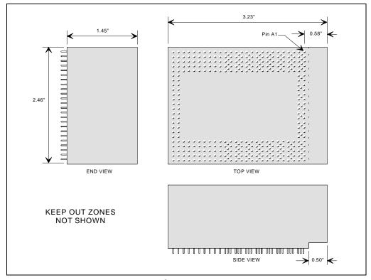
Figure 17-3. OverDrive® Processor Envelope Dimensions
