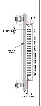
Figure 17-5. Header 8 Pinout
