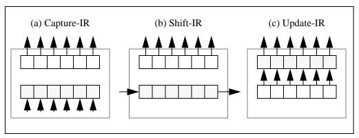
Figure 10-4. Operation of the Pentium® Pro Processor TAP Instruction Register
