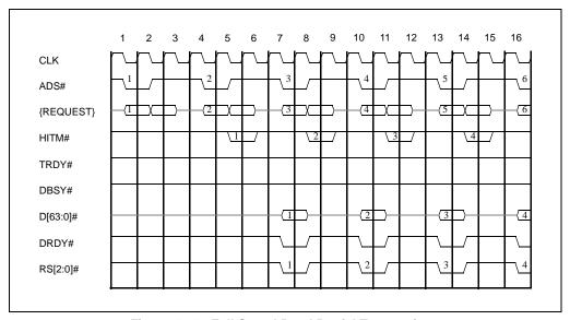
Figure 4-21. Full Speed Read Partial Transactions
