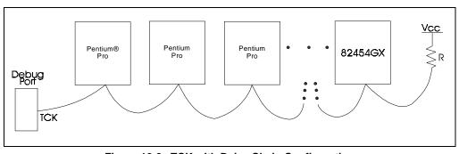
Figure 16-2. TCK with Daisy Chain Configuration
