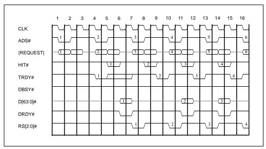
Figure 4-24. Full Speed Write Partial Transactions
