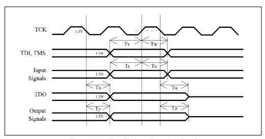
Figure 11-14. Test Timings (Boundary Scan)
