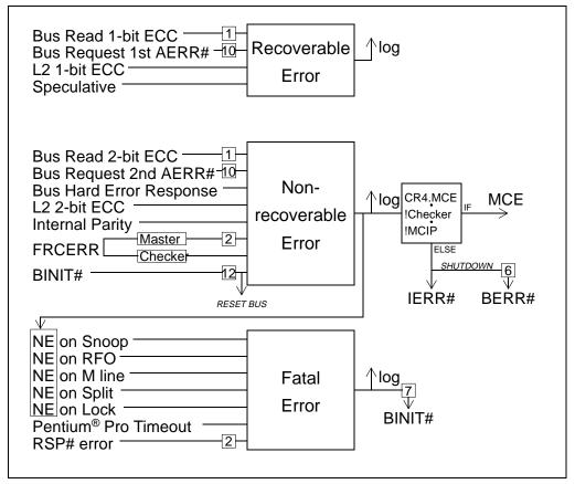
Figure 8-3. Pentium® Pro Processor Errors
