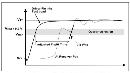
Figure 12-7. Extrapolated Flight Time of a Non-Monotonic Rising Edge
