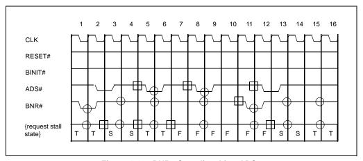
Figure 4-10. BNR# Sampling After ADS#
