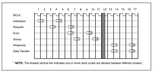
Figure 3-2. Pentium® Pro Processor Bus Transaction Phases
