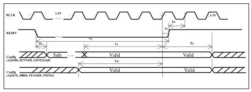
Figure 11-12. Reset and Configuration Timings
