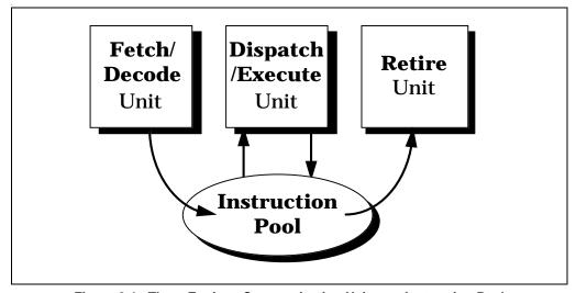
Figure 2-1. Three Engines Communicating Using an Instruction Pool
