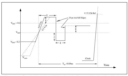
Figure 12-3. Standard Input Lo-to-Hi Waveform for Characterizing Receiver Ringback Tolerance
