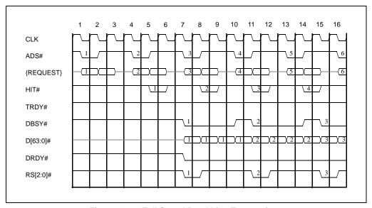
Figure 4-23. Full Speed Read Line Transactions
