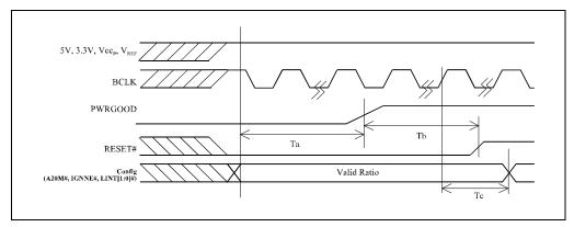
Figure 11-13. Power-On Reset and Configuration Timings
