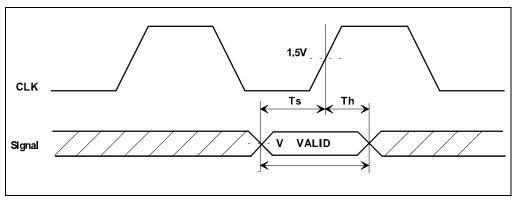
Figure 11-9. Setup and Hold Timings
