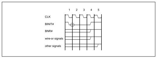
Figure 4-3. Signal Deassertion After Bus Reset
