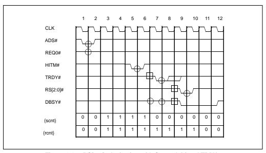
Figure 4-16. RS[2:0]# Activation with Snoop Initiated TRDY#
