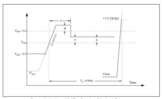
Figure 11-10. Lo to Hi GTL+ Receiver Ringback Tolerance
