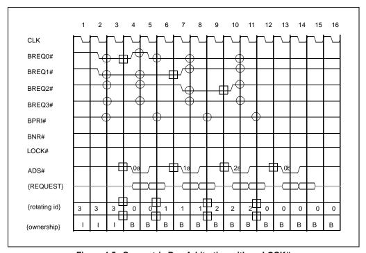
Figure 4-5. Symmetric Bus Arbitration with no LOCK#
