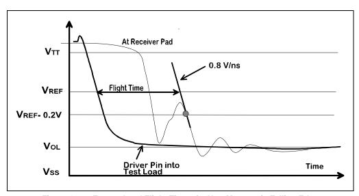
Figure 12-8. Extrapolated Flight Time of a Non-Monotonic Falling Edge
