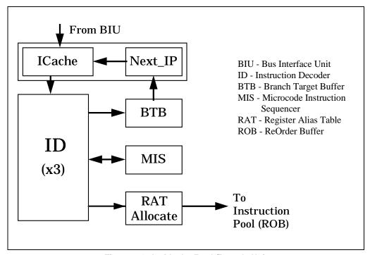
Figure 2-4. Inside the Fetch/Decode Unit
