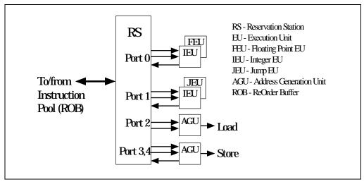
Figure 2-5. Inside the Dispatch/Execute Unit
