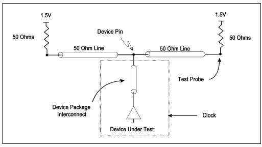
Figure 12-11. Test Load for Measuring Output AC Timings
