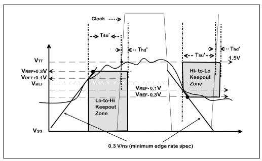
Figure 12-10. Unacceptable Signal, Due to Excessively Slow Edge After Crossing  $V_{\mathsf{REF}}$
