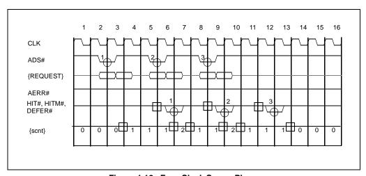
Figure 4-12. Four-Clock Snoop Phase
