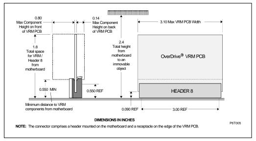
Figure 17-6. OverDrive® Voltage Regulator Module Envelope
