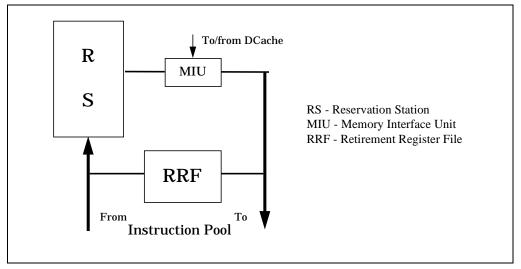
Figure 2-6. Inside the Retire Unit
