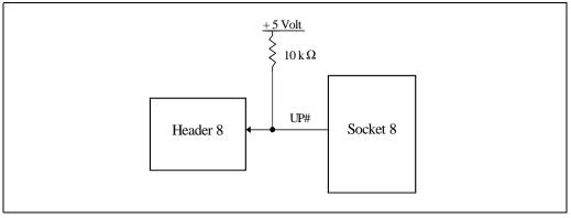
Figure 17-7. Upgrade Presence Detect Schematic - Case 1
