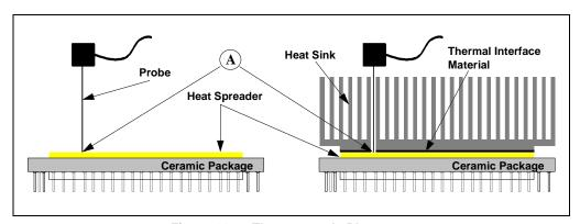
Figure 14-2. Thermocouple Placement
