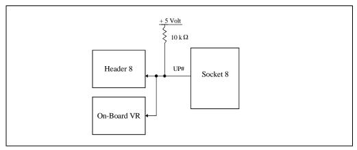
Figure 17-8. Upgrade Presence Detect Schematic - Case 2
