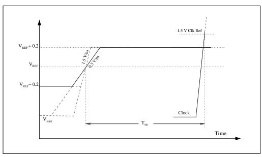
Figure 12-13. Standard Input Lo-to-Hi Waveform for Characterizing Receiver Setup Time
