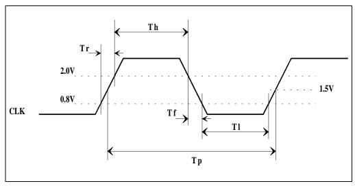
Figure 11-7. Generic Clock Waveform
