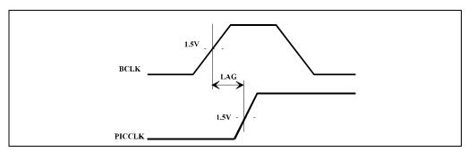
Figure 11-11. FRC Mode BCLK to PICCLK Timing
