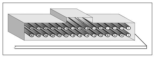
Figure 16-5. Debug Port Connector on Primary Side of Circuit Board
