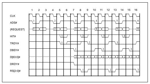
Figure 4-25. Full Speed Write Line Transactions
