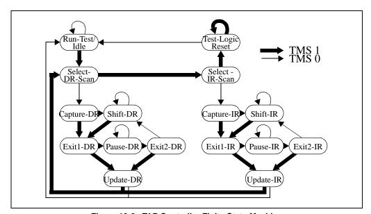
Figure 10-2. TAP Controller Finite State Machine
