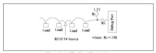
Figure 16-1. GTL+ Signal Termination
