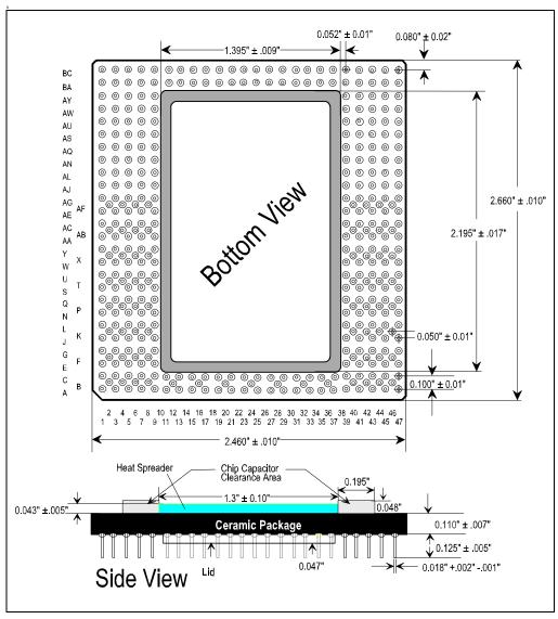
Figure 15-1. Package Dimensions-Bottom View
