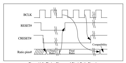
Figure 11-3. Timing Diagram of Clock Ratio Signals
