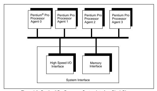
Figure 1-2. Pentium® Pro Processor System Interface Block Diagram
