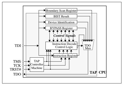
Figure 10-1. Simplified Block Diagram of Pentium® Pro Processor TAP logic
