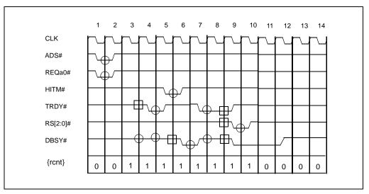
Figure 4-17. RS[2:0]# Activation After Two TRDY# Assertions
