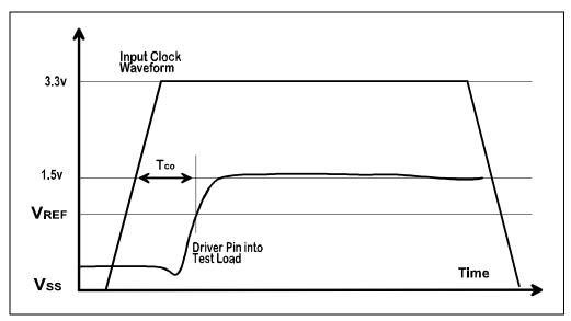
Figure 12-12. Clock to Output Data Timing (T<sub>CO</sub>)
