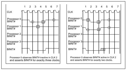
Figure 8-2. BINIT# Protocol Mechanism
