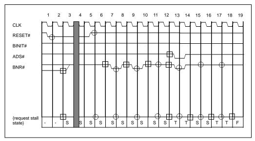
Figure 4-9. BNR# Sampling After RESET#
