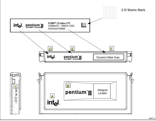
Figure 36. S.E.C. Cartridge Mark Locations
