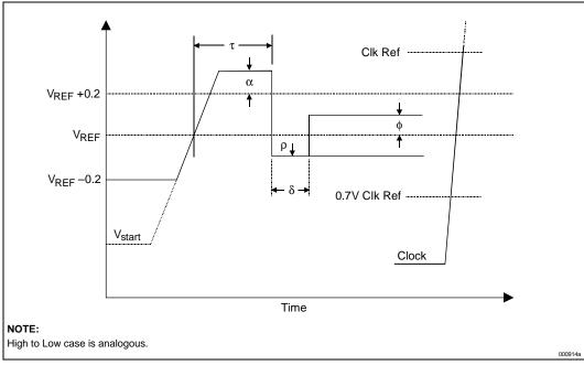
Figure 16. Low to High GTL+ Receiver Ringback Tolerance
