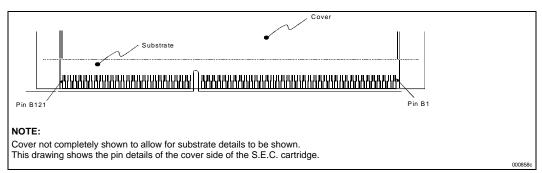
Figure 39. S.E.C. Cartridge Substrate Dimensions, Cover Side View
