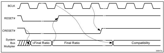
Figure 4. Timing Diagram of System Bus Multiplier Signals
