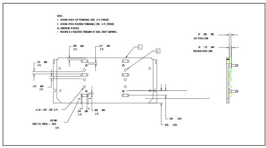
Figure 28. Heatsink Attachment Mechanism Design Space
