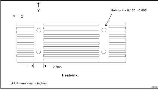
Figure 27. General Rivscrew\* Heatsink Mechanical Recommendations
