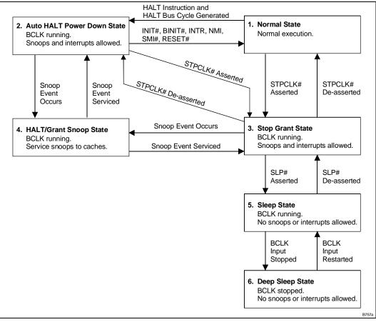
Figure 3. Stop Clock State Machine
