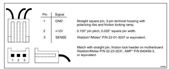
Figure 48. Boxed Processor Fan/Heatsink Power Cable Connector Description
