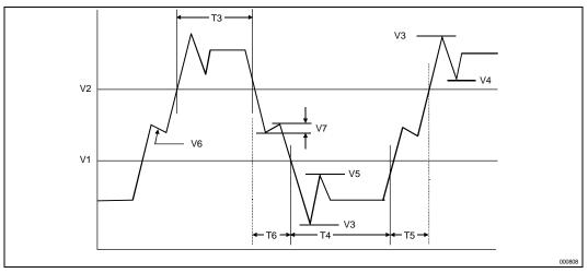
Figure 15. BCLK, TCK, PICCLK Generic Clock Wave form at the Processor Edge Fingers
