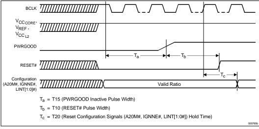
Figure 12. Power-On Reset and Configuration Timings
