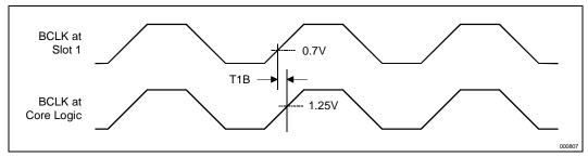
Figure 6. BCLK to Core Logic Offset
