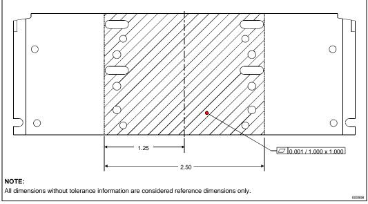
Figure 33. S.E.C. Cartridge Thermal Plate Flatness Dimensions
