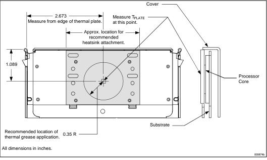
Figure 19. Processor Thermal Plate Temperature Measurement Location
