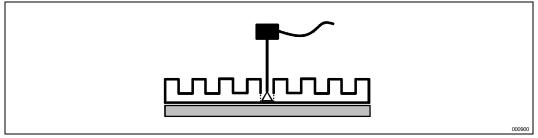
Figure 21. Technique for Measuring TPLATE with 90° Angle Attachment
