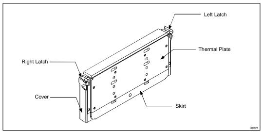
Figure 18. Processor S.E.C. Cartridge Thermal Plate
