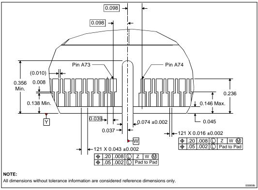
Figure 40. Substrate – S.E.C. Cartridge Substrate Detail A
