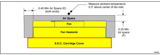
Figure 44. Top View Space Requirements for the Boxed Processor
