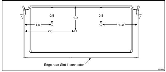
Figure 22. Guideline Locations for Cover Temperature (T<sub>COVER</sub>) Thermocouple Placement
