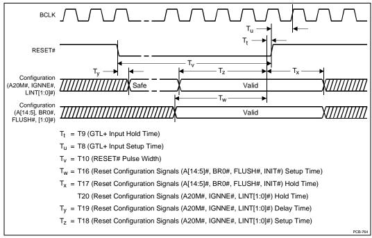
Figure 11. System Bus Reset and Configuration Timings
