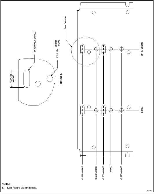
Figure 32. S.E.C. Cartridge Thermal Plate and Side View Dimensions
