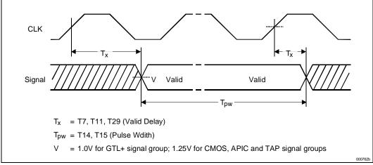
Figure 8. System Bus Valid Delay Timings
