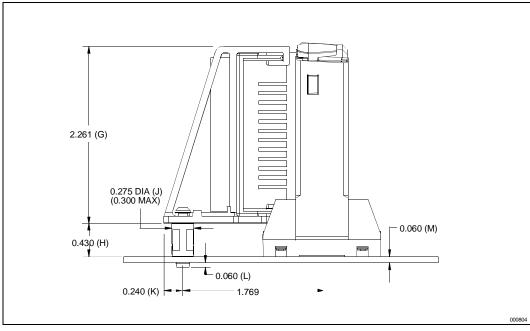
Figure 46. Side View Space Requirements for Boxed Processor Fan/Heatsink Supports
