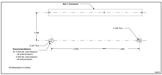
Figure 45. Heatsink Support Hole Locations and Sizes
