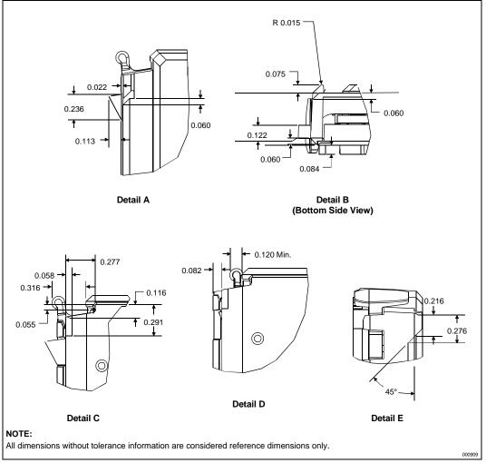
Figure 34. S.E.C. Cartridge Latch Details
