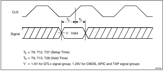
Figure 9. System Bus Setup and Hold Timings
