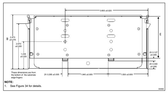
Figure 31. S.E.C Cartridge Thermal Plate Side Dimensions
