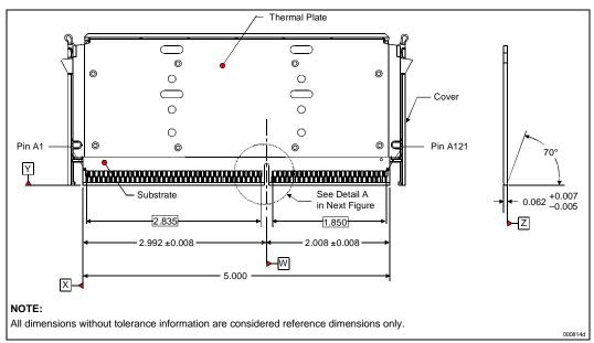
Figure 38. S.E.C. Cartridge Substrate Dimensions
