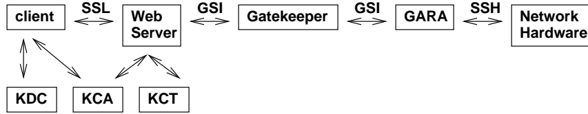
Figure 6.2: KX509 GARA Web Interface. This figure shows how local network resources are reserved with the GARA Web interface. KX509 junk keys replace long term PK credentials.
