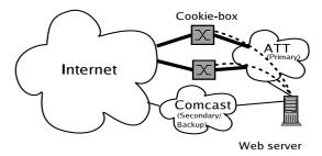
Figure 2: A multihomed web server seeking protection deploys cookie boxes at some of the network links of its primary ISP. These could be edges along which the web server expects to receive a large fraction of its traffic.
