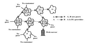
Figure 1: ISPs shaded gray are in the region of trust of the web server. ISPs enclosed in a white square are on the trust boundary For example, ISPs A and B are on the trust boundary since they terminate the trust chain for traffic received from their peers.
